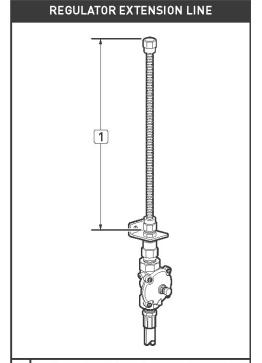
Factory installed regulator extension line is 305mm (12") long. Do not replace with longer line.
