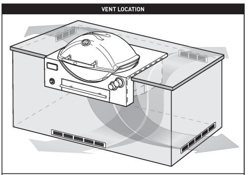
A minimum of 254 square cm (100 square inches) of venting per side on at least two sides of the structure is recommended.
