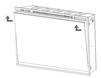
NOTE: PLEASE DO NOT LIFT THE GLASS UP BY LIFTING THE "U" SHAPE METAL BRACKET.
