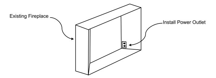
**NOTE:** A dedicated 10 Amp (or higher) breaker is required. This fireplace must be electrically connected and grounded in accordance with local codes.
