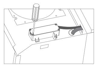
**7.** Connect the wire as following picture show, then close the box cover and fix it with screws.
