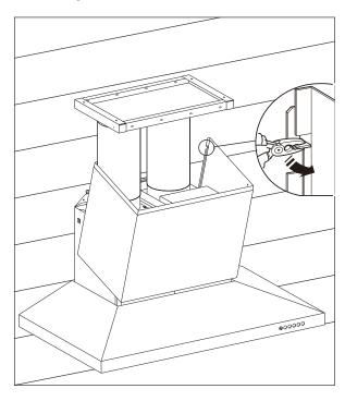
**10.** Slide telescopic flue cover to upper position and fix with screws provided.
