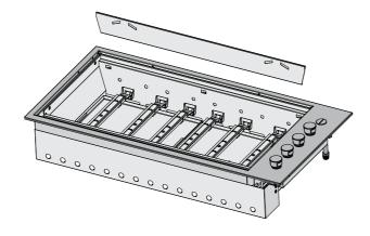
3. Install flame tamers (under grills) and fix back edge of flame tamer into the heat shield panel.
