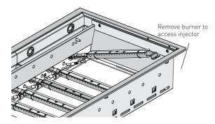
Unscrew Natural gas injectors and replace with either Universal LPG or Propane injectors. Universal LPG injectors have 0.90mm diameter orifice. Propane Gas injectors have 0.95mm diameter orifice. All injectors are marked with the orifice size.
