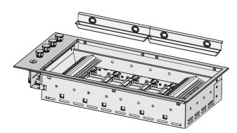
5. Install hotplates and grills as shown, ensuring that the flame tamers are located under the grills.
