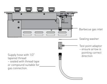
After connecting the barbecue to an Universal LPG gas supply, test the operation of the appliance:
