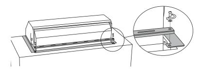
The front cover can be removed for accessing the Fat-Collecting Pan and replaced:
