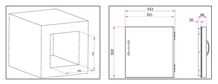
NOTE: The cutout of each corner should be 90° angle in order for the access door to fit properly.
