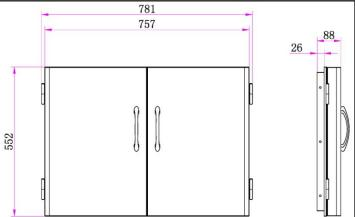
**NOTE:** The cutout of each corner should be 90° angle in order for the unit to fit properly.
